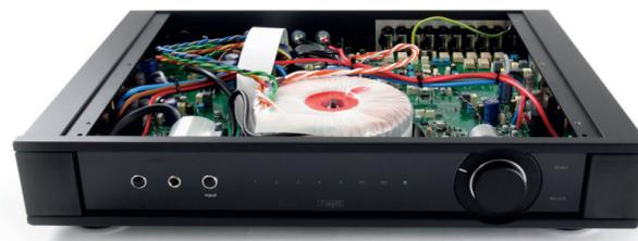
High-quality relays, Sanken output transistors, discrete circuitry, and polypropylene capacitors are used throughout the amp design
