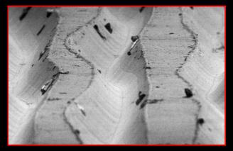
Towards the centre of an LP, a 10Khz signal is just 26 microns long and if it's very quiet it may be less than 10 microns high. If your tonearm has 10 microns of movement within the bearing assemblies (and even very expensive tonearms usually have much more play and movement), reading the bumps will be difficult and musical vibration will be lost in arm movement.
