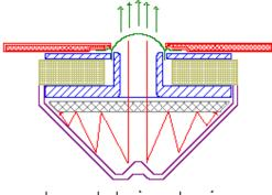
Large hole in pole piece Small amount of damping and No reflection
