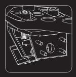
Using incorrect bolts will destroy the fine wires inside the cartridge.
