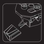
Carefully re-fit the stylus guard after each use. Avoid touching the stylus.
